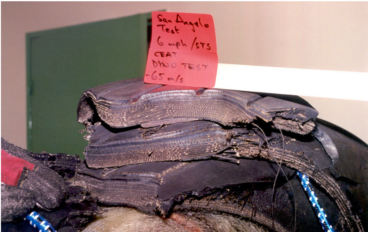
Figure 50: Cuts in various Concorde tyres
