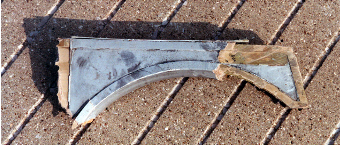
Figure 19: Part located at line 157 - right part of deflector
